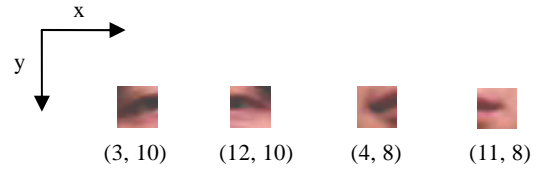
Figure 11 . The template images and values of feature points (right eye side, left eye side, right lip corner, left lip corner)
