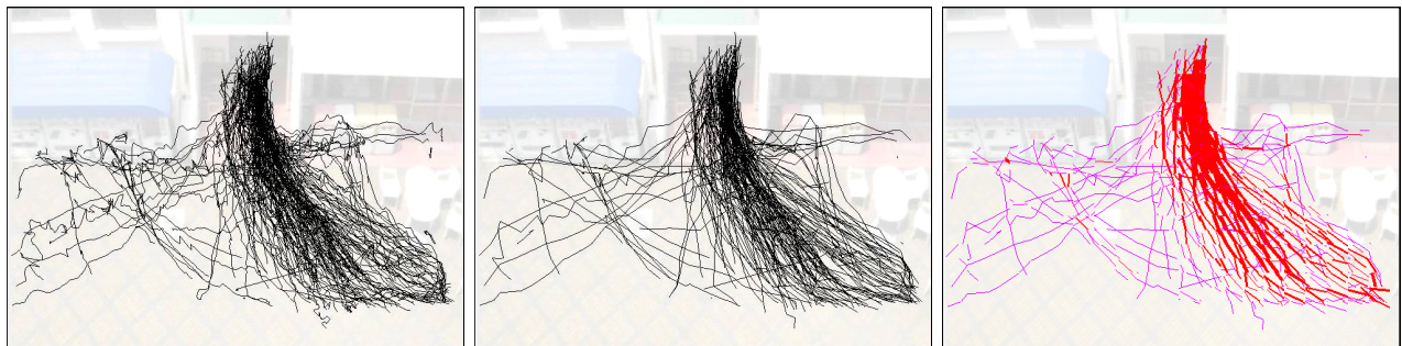
Figure 6. Rendering segments of the paths captured from a movie file. (Left) The technique renders corresponding one segment as is. (Center) The technique calculates intersections between segments and grids, connects the intersections by straight segments, and renders the segments. (Right) The technique calculates the average of the corresponding segments, and renders according to relative density.
