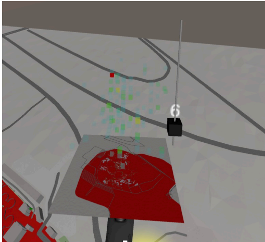
Fig. 5. MiniMap views the time change of the number of the tweets in a day. Cubes in MiniMap indicate the aggregation of one-hour data different from those in WorldView. Users can observe the time change more specifically.
